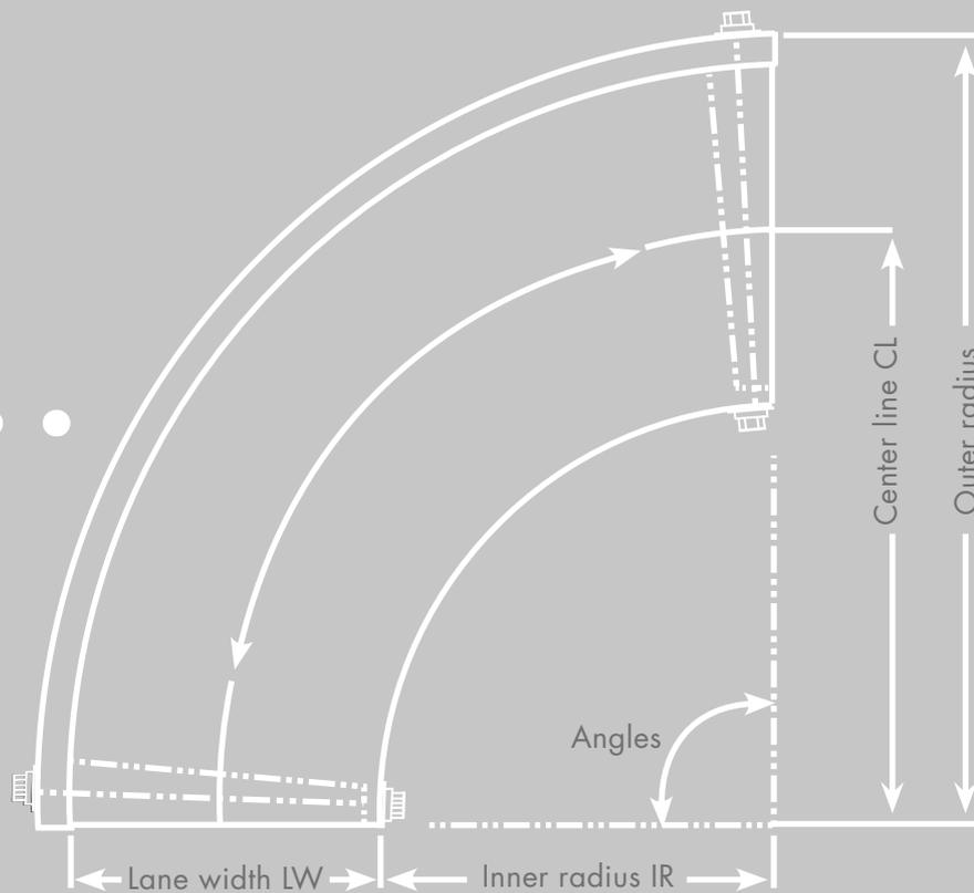
Conventional, friction driven belt curves frequently present the problem of belt slippage and, as a result, overheating of the belt:
