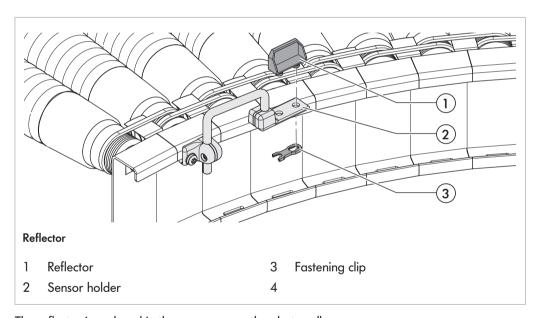
The reflector is replaced in the same way as the photo cell:
