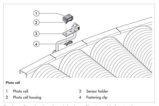
The photo cell is replaced together with the photo cell housing and the fastening clip:
