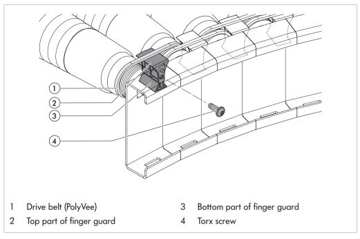
The finger guard protects against injuries as well as damage to the belt.
