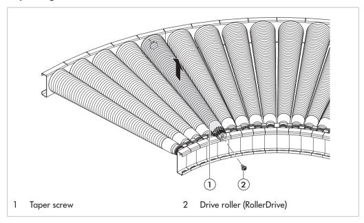
Replacing the RollerDrive is required only if the roller is damaged, or the drive is defective.
