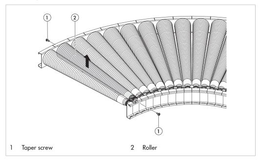
Replacing the roller is only necessary if the PolyVee heads show signs of wear or the roller is damaged.
