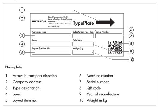
The information on the nameplate is used to identify the conveyor. The type designation is required to use the conveyor according to its intended use.
