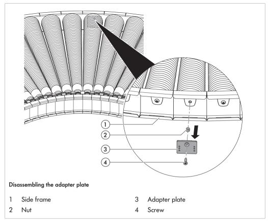
▶ If the MultiControl is to be completely disassembled or the adapter plate to be replaced, also loosen the screw (4) with which the adapter plate (3) is fastened at the side frame (1) and remove adapter plate with nut (2) from the side frame.
